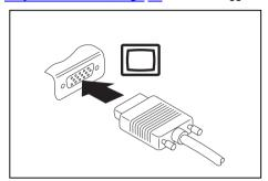
Analogue VGA monitor connection socket
